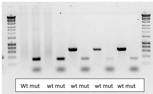
Separated by gel electrophoresis on a 2% agarose gel.
