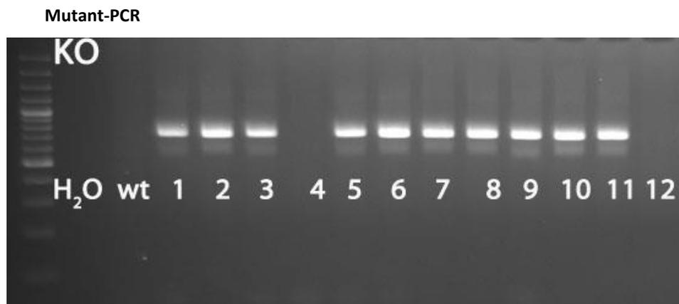
Separated by gel electrophoresis on a 2% agarose gel.
