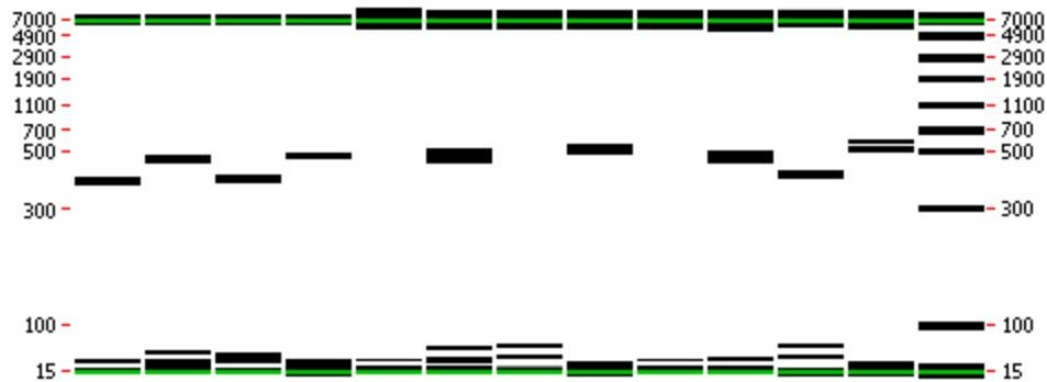
Note that as this technology is more sensitive than gel analysis, non specific signals and/or primer dimers may be visible on the picture.
