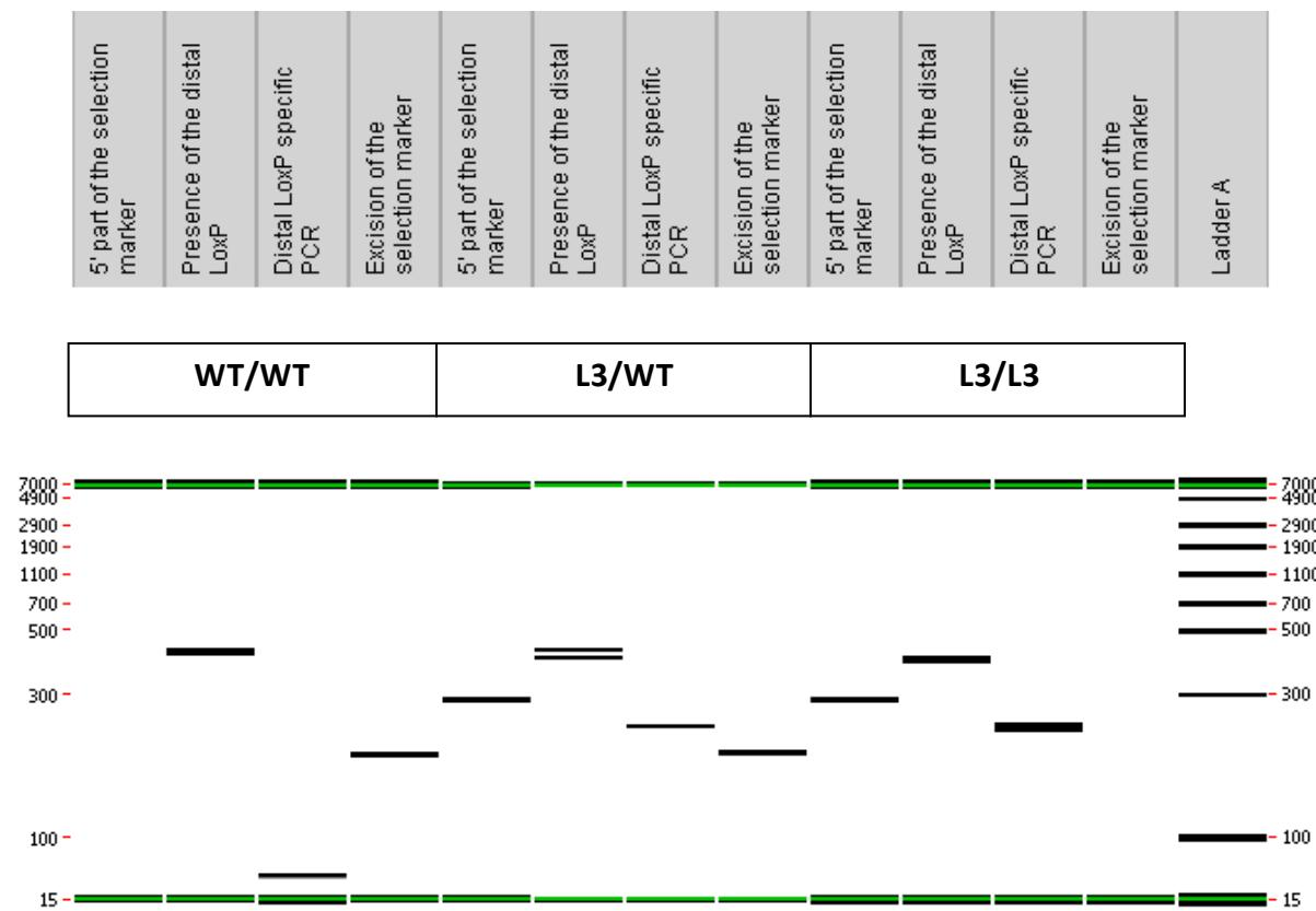
Note that as this technology is more sensitive than gel analysis, non specific signals and/or primer dimers may be visible on the picture.
