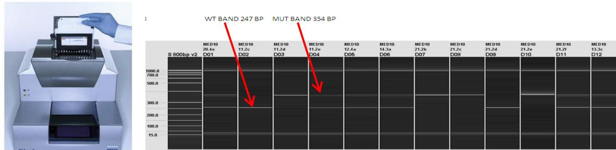
PCR is performed using KAPA2G Fast Hotstart Readymix (2X), although alternatives may be used.
