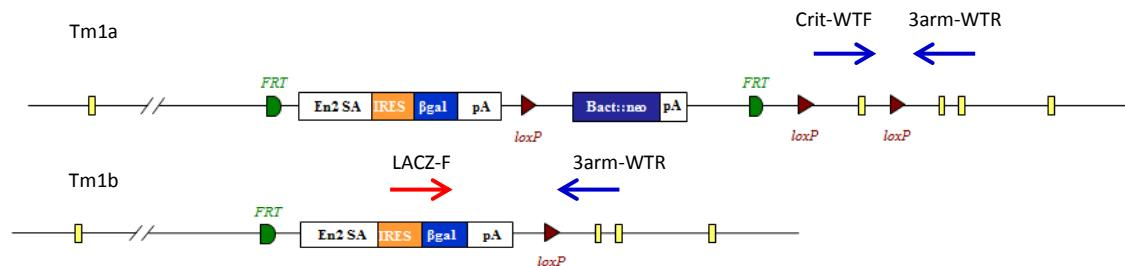
If the deletion of the critical region has not occurred then a product is produced between the -Crit-WTF and the -3arm-WTR. Complete conversion by Cre will mean a product is produced from the LacZ-F and -3arm-WTR as the two primers now lie close enough to generate a PCR product under standard conditions. Run both the tm1a genotyping protocol to detect WT and tm1a alleles and the tm1b protocol to detect converted alleles.
