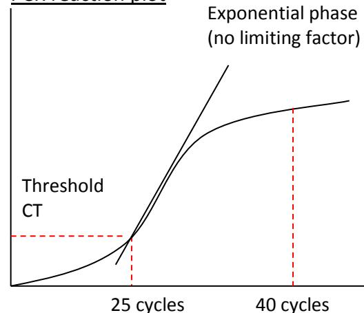
The number of cycles the PCR takes to reach a set threshold is known as the CT value. This is inversely correlated to the amount of template DNA in the sample.
