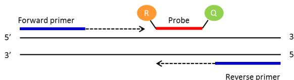
As the forward primer is extended the reporter is cleaved from the probe resulting in a fluorescent signal being detected. Once the primer extends enough to release the quencher this signal is blocked. By using probes with different fluorescent signals multiple PCR assays can be multiplexed and run together.
