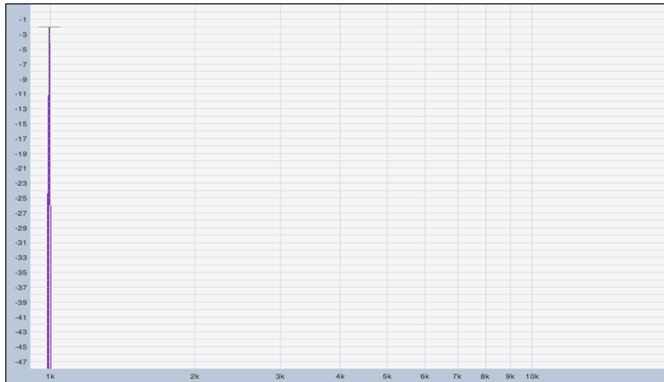
1kHz pure tone just below clip level (Vertical = level in decibels, horizontal = frequency)
