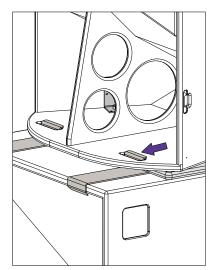
Slide the Evo X forwards to engage the cabinet with the clasps.
