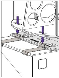
Lower the Evo X onto the board, passing the hooks of the 2x ClaspLD through the cutouts in the cabinet.
