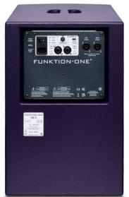
Frequency Response (-3dB): 45Hz - 300Hz Weight: 19kg (42lbs) Power output (8 $\Omega$ ): 1x 300W (LF) 2x 75W (Satellites) Minimum load impedance: 4 $\Omega$  (Satellites) Active crossover: 130Hz 24dB Linkwitz-Riley AC Power: 100-240VAC 50-60Hz 120W
